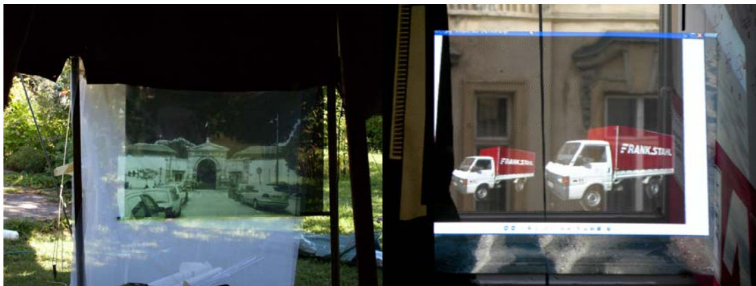
Figure 78: Improved screen material versus metal screen
